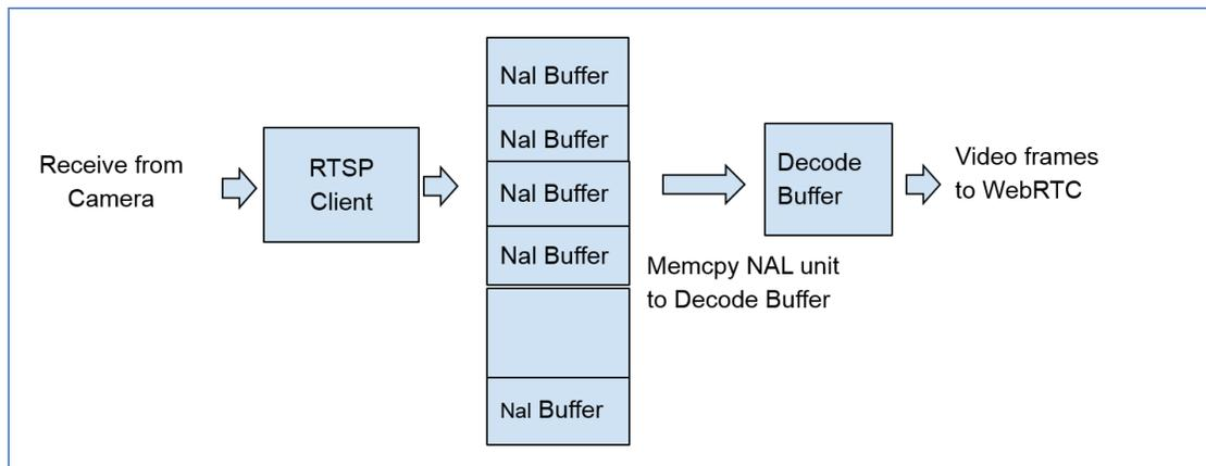
For the media gateway implementation, the WebRTC encoder output is overridden with the H.264 frames from RTSP. The encoder works on its input from camera. The output is packed in to RTP and sent over webRTC. We override the contents of the encoder to insert video frames from RTSP. This way, the need for decoding and re-encoding the media is avoided and the program runs more efficiently.
