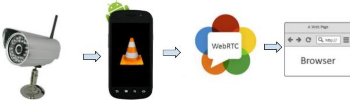
A media Gateway can be implemented using the RTSP client and WebRTC implementations in the host platform. However, there is a significant amount of customization needed to do this, as the default WebRTC implementation typically supports only the built-in camera of the system. For example, WebRTC implementation on Android supports only its on-board cameras. There are two ways the media can be bridged between RTSP and WebRTC.
