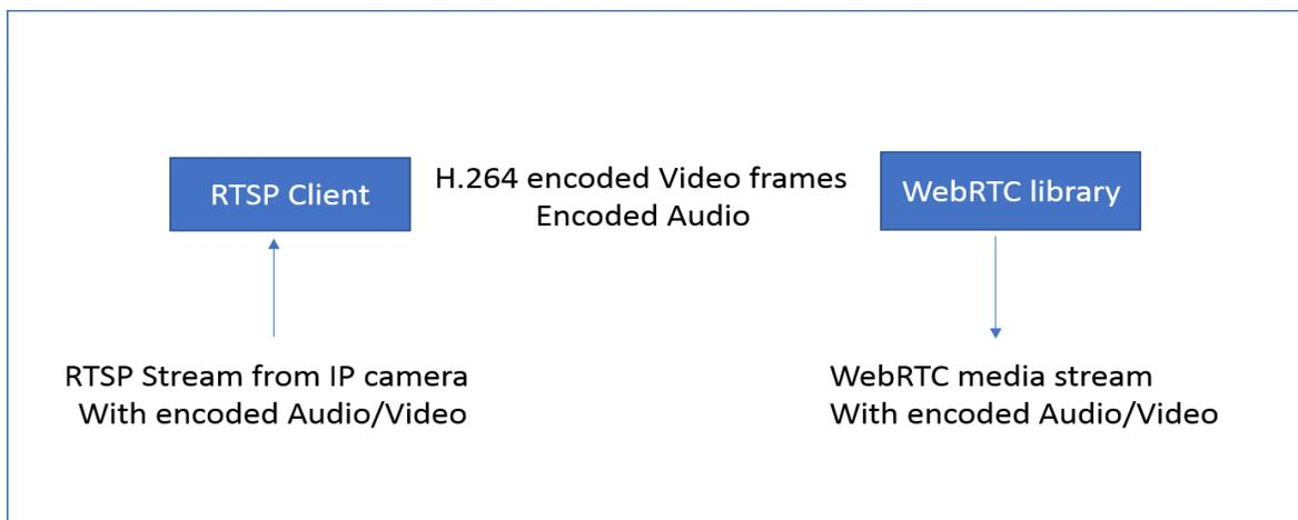
Implementing media forwarding involves video frame capture, video stream processing and playing the video on the WebRTC. Details on these topics are given in the sections below.
